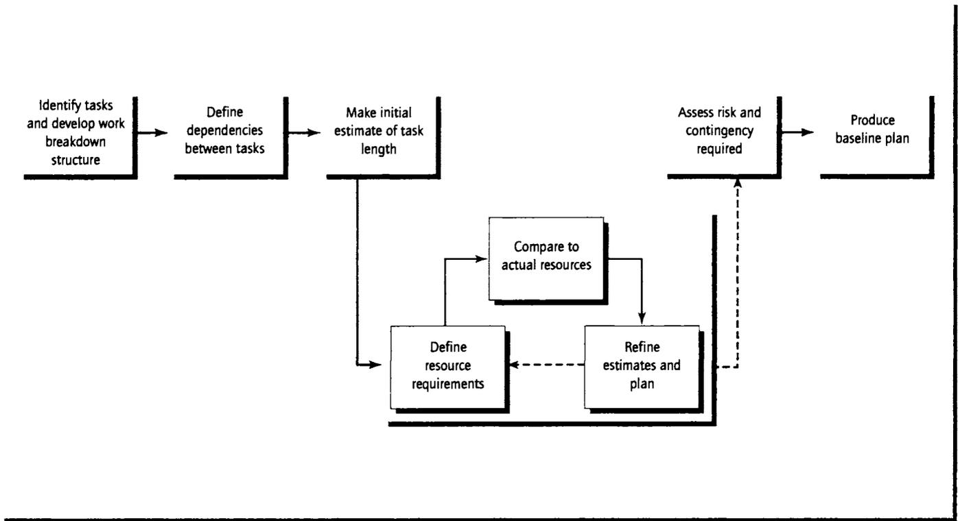
**figure 5.1** Developing a project plan
